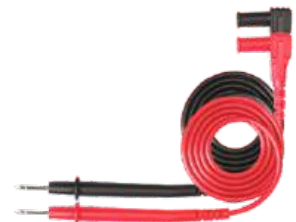
H3004 Probe:Length 90mm ,TipΦ2mm Plug:Φ4mm 90 degree bend plug Wire:24WG,red/black Length:800mm Safety Class:EN61010-031,1000V CATII
