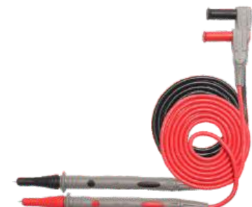
H3006 Probe:Length 130mm,TipΦ4mm Banana Plug:Φ4mm 90 degree bend plug Wire:18AWG,red/black Length:1200mm Safety Class:EN61010-031,1000V CATIII/600V CATIV,MAX 10A
