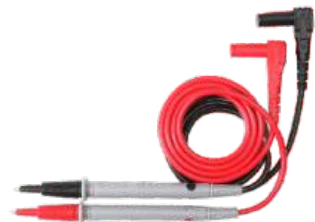
H3002 Probe:Length 120mm,TipΦ2mm Plug:Φ4mm 90 degree bend plug Wire:22AWG,red/black Length:800mm Safety Class:EN61010-031,1000V CATII,MAX 10A
