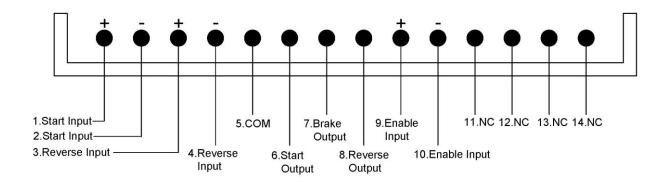
Please find the 14 Pin connector on top of the controller box and follow the input and output control functions wiring:
