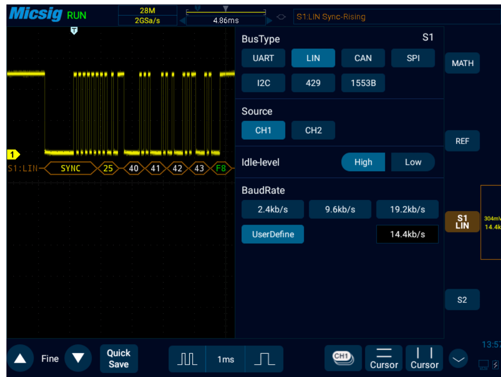
Figure 12-10 LIN Bus Configuration Menu
