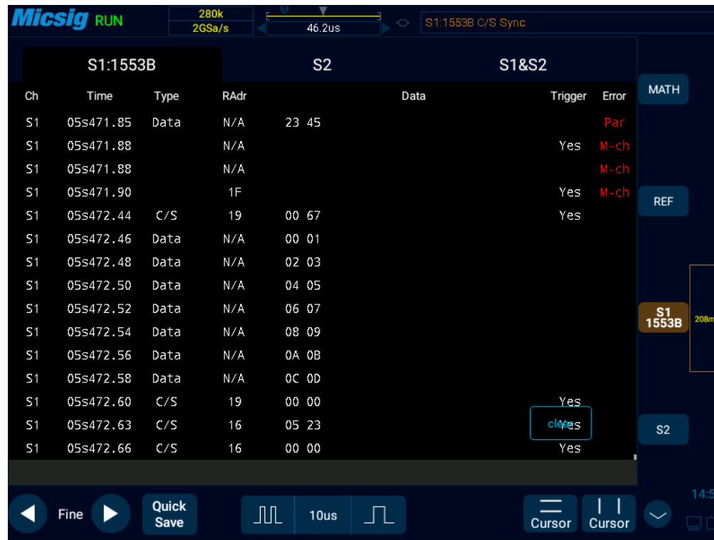
Figure 12-33 1553B Text Interface
