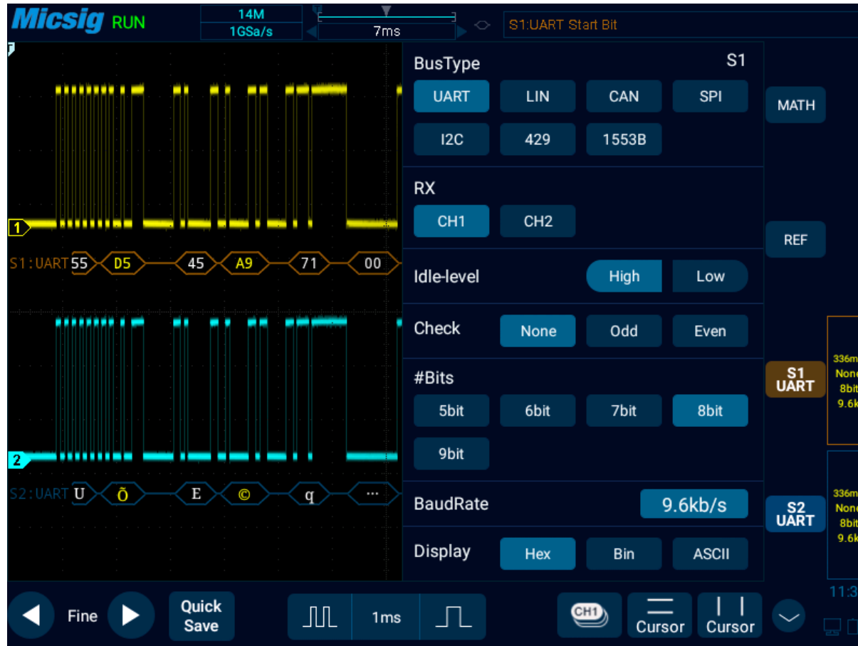
Figure 12-1 Bus Type Selection Menu
