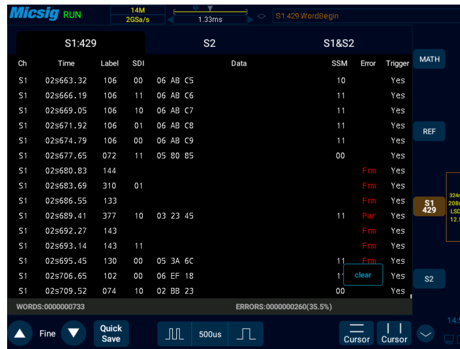
Figure 12-29 ARINC429 Text Interface
