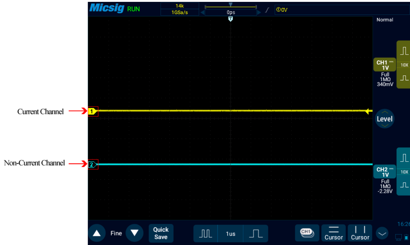
Figure 5-2 Current Channel and Non-Current Channel
