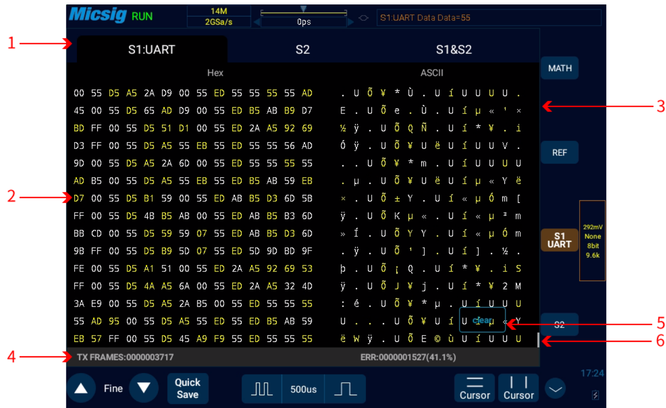
Figure 12-9 UART Text Interface
