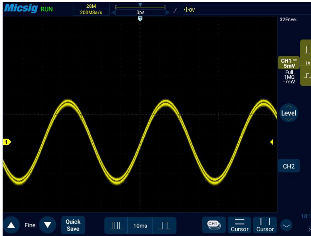
Figure 11-8 AM Signal in Envelope Sampling Mode (32)
