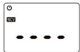
2) Press NCV key, put the NCV sensor close to the measured cable, the meter could detect if the measured cable is >90V AC voltage or not. When the meter detects AC voltage, the meter buzzer alarms and the backlight flashes.
