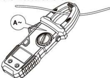
3 ) When measuring the current, when capture current >10.0A, the meter displays the maximum current value captured.
