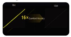
12-bit vertical resolution provides 4096vertical digitizing levels16 times the vertical digitizing level of the8-bit resolution
