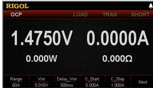
Figure 2-30 Main Interface of OCP Test Function
