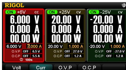
Figure 2-13 Timing output (normal display mode)
