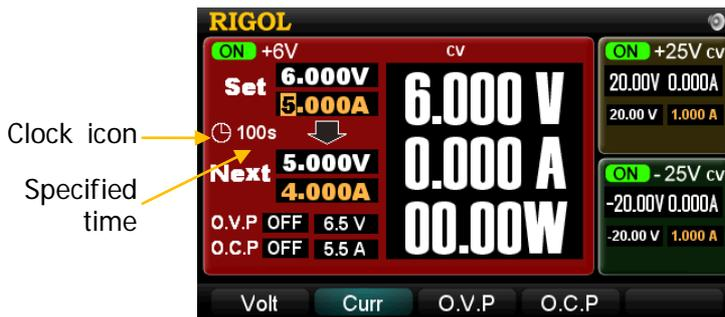
Figure 2-12 Timing output (in focus display mode)
