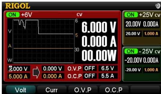
Figure 1-8 Focus waveform display mode
