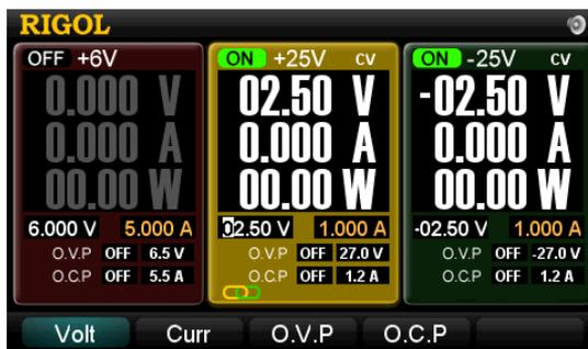
Figure 2-17 Tracking output (after tracking)
