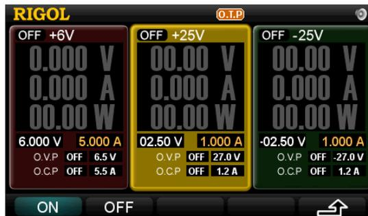
Figure 2-28 Over-temperature Protection Settings
