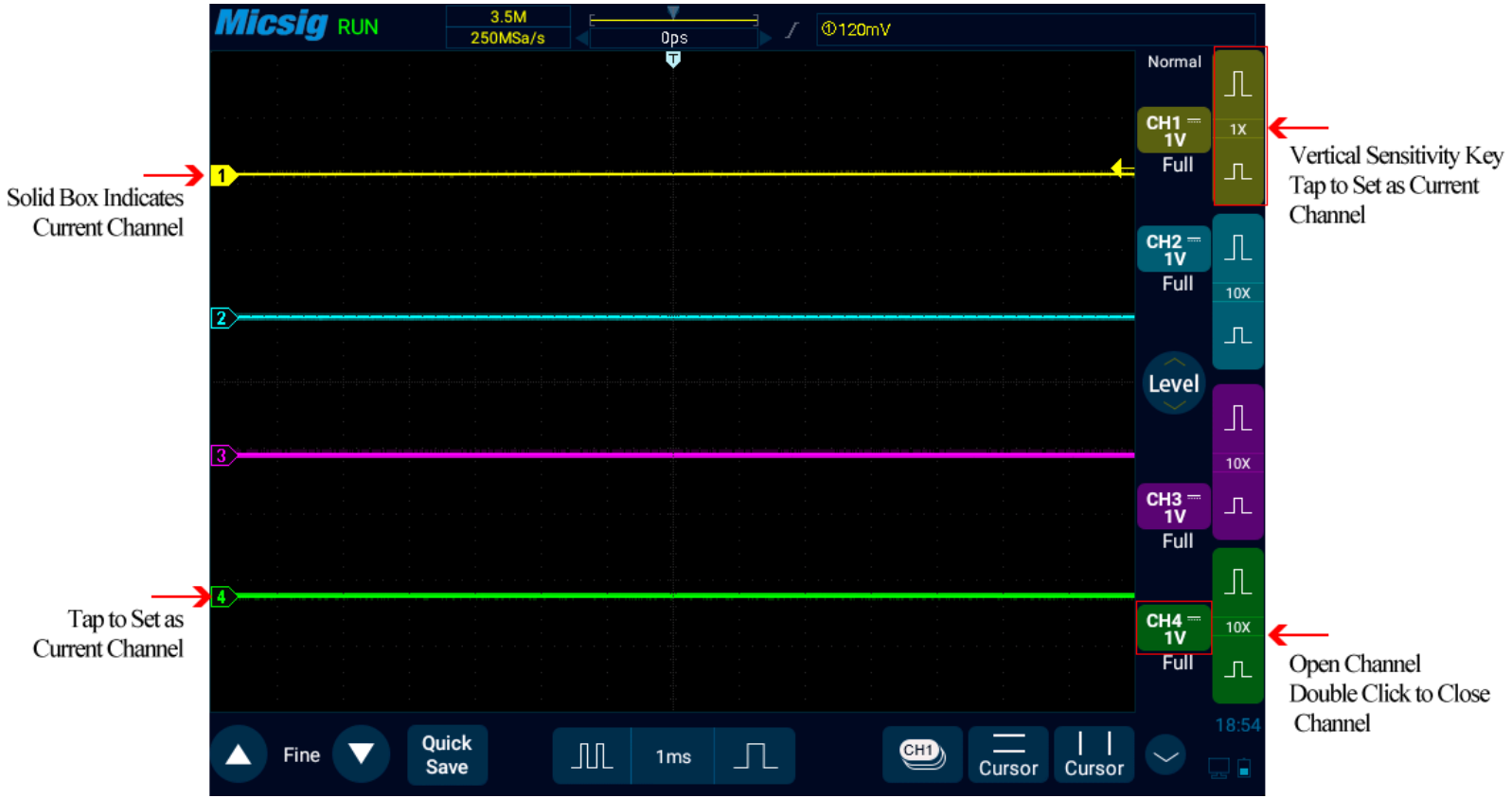
Figure 5-4 Channel Open, Close and Switching
