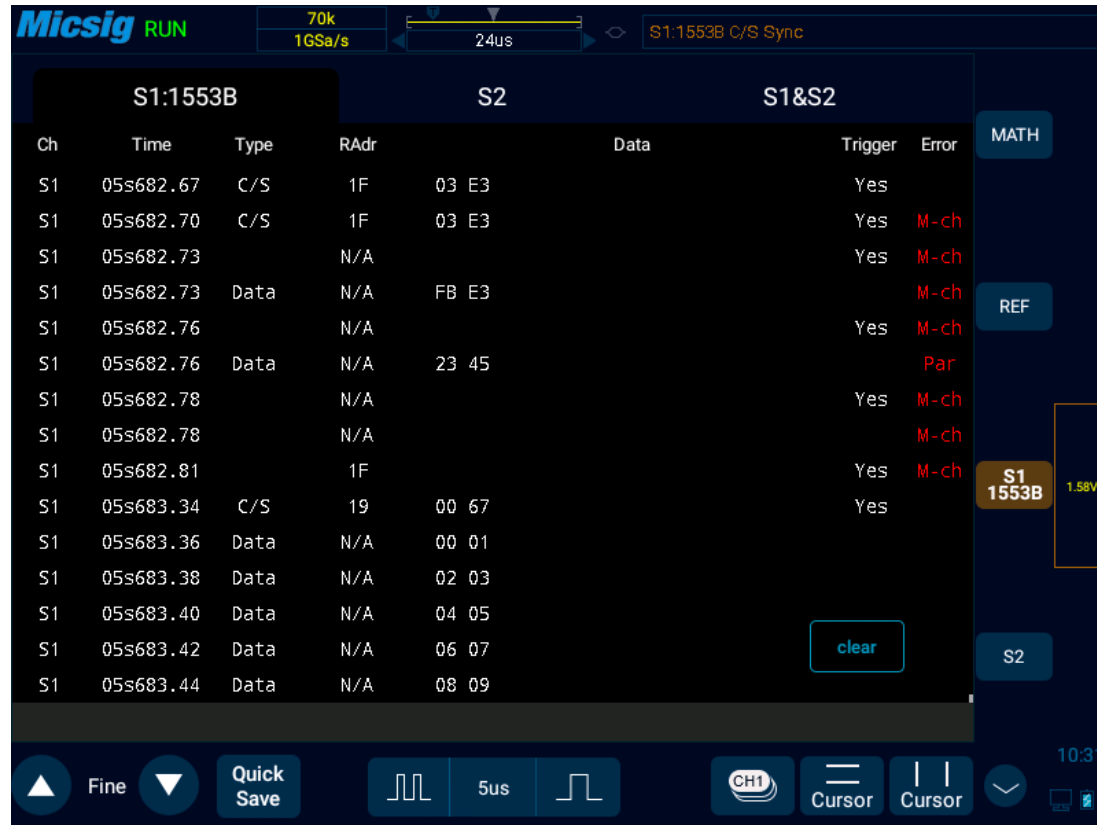
Figure 12-33 1553B Text Interface
