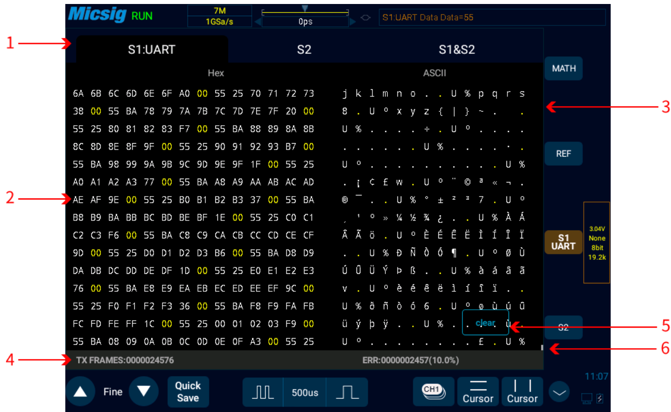
Figure 12-9 UART Text Interface
