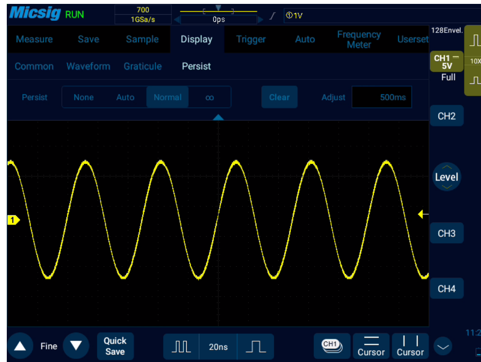
Figure 10-4 20MHz Sine Wave Variable Persistence 500ms
