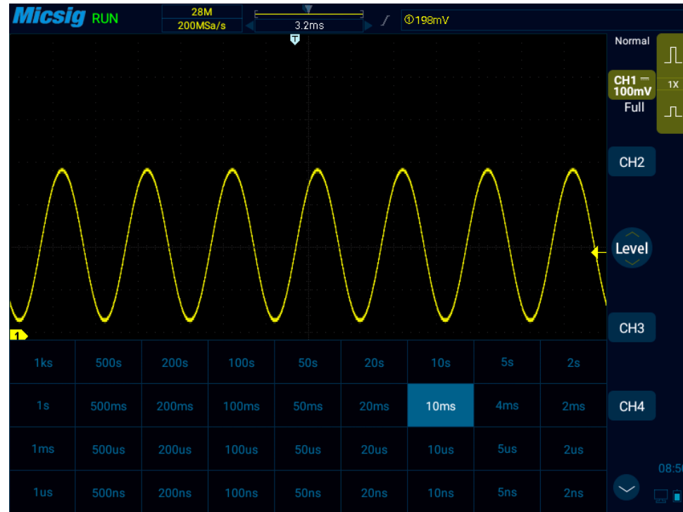
Figure 4-4 Horizontal Time Base Knob
