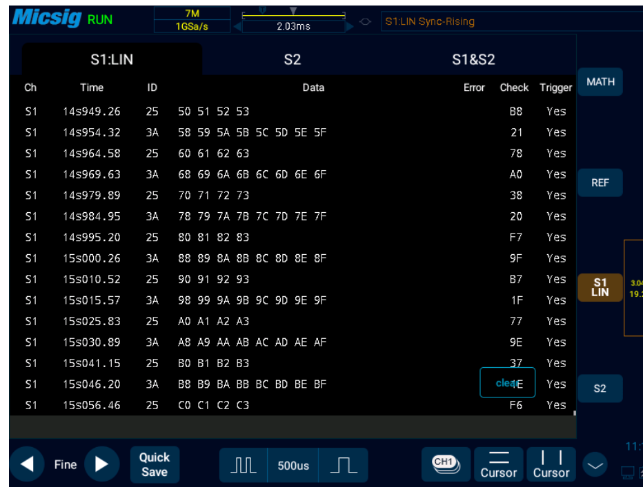
Figure 12-13 LIN Text Interface
