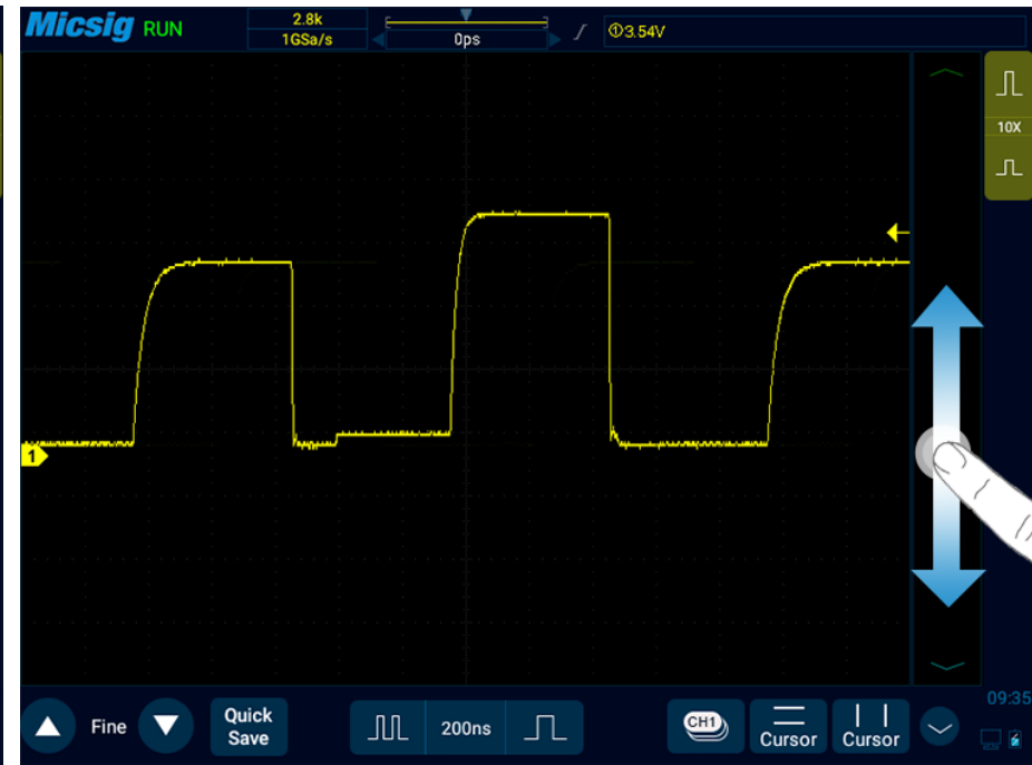
Figure 6-4 Abnormal Signal Captured by Setting Trigger Level
