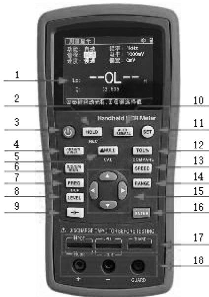
Figure 1 Front panel (with “100k Continuous Fr. Type” as an example)
