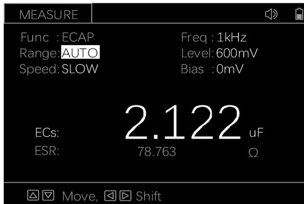
Fig 12 Electrolytic capacitance mode
