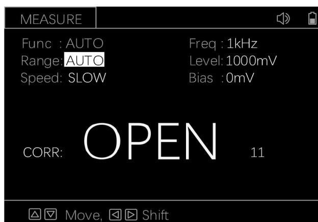
Fig 15 Open circuit correction
