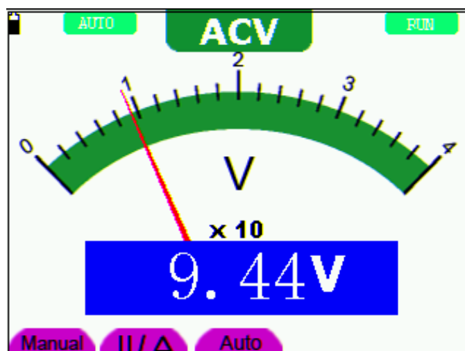
figure 26: AC Voltage Measurement
