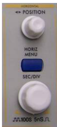
Fig. 10 Horizontal Control Zone
